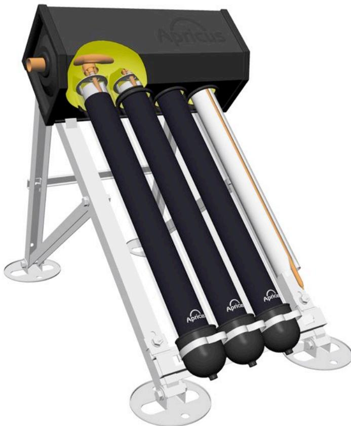
Apricus has perfected the design of a copper heat pipe to effectively conduct the heat from within the evacuated tube up to an insulated header box. A dry connection between the heat pipes and the heat exchanger means that the heat pipe is not in contact with the water, and so there are no seals to fail. It also makes the installation “plug and play”, greatly reducing the time the plumber has to spend on the roof.
